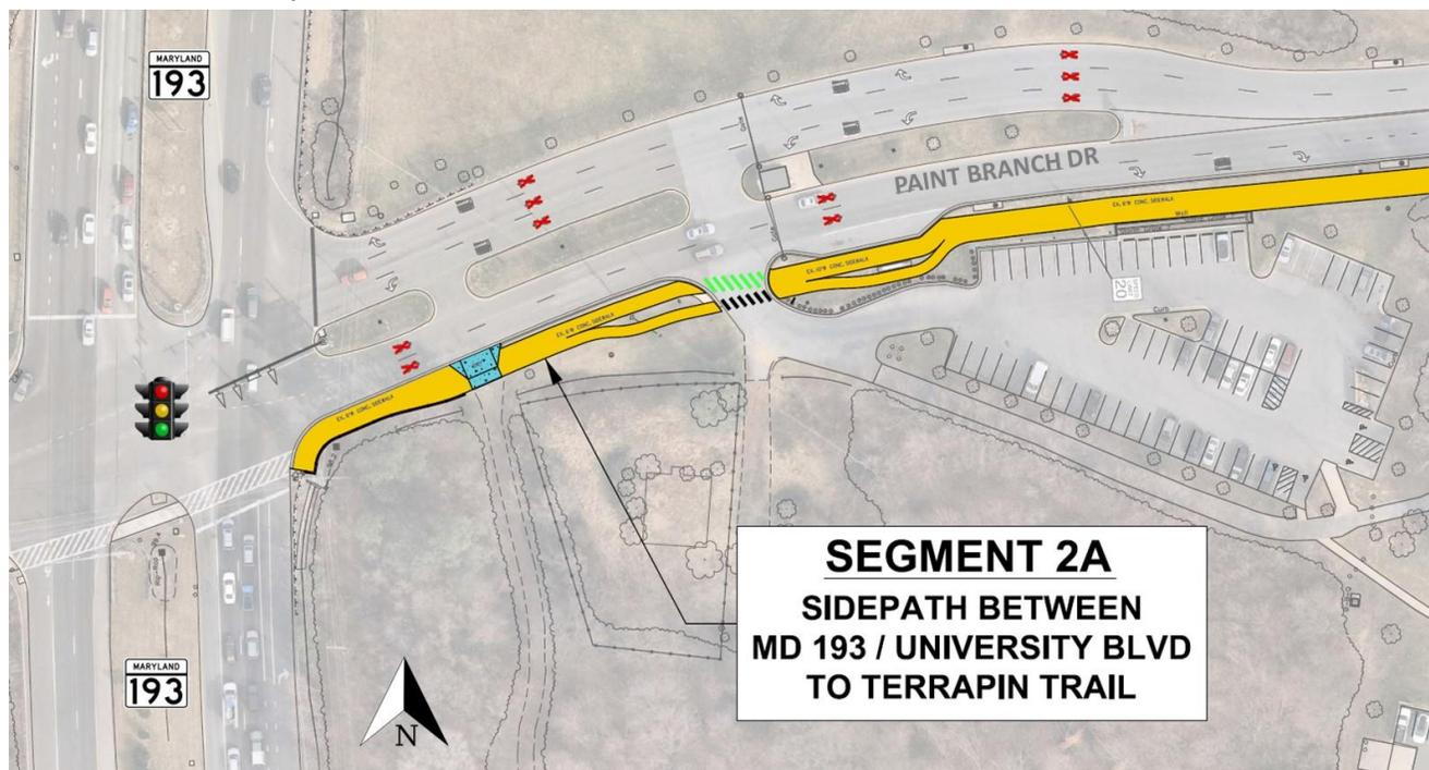
FIGURE 23: PROPOSED SIDE PATH ALONG SOUTH SIDE OF PAINT BRANCH DR NEAR MD 193
