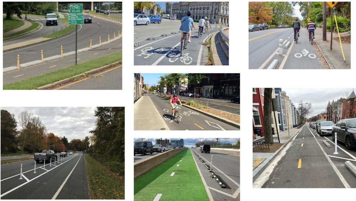
FIGURE 4: VARIOUS ON-ROAD CYCLETRACK VERTICAL PROTECTION ELEMENTS
