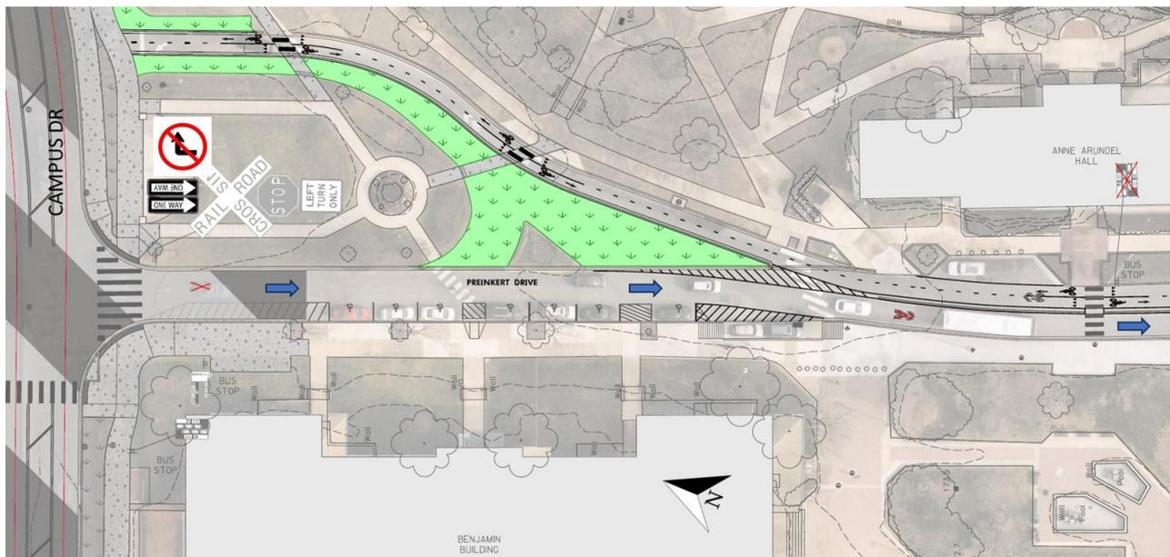
FIGURE 21: PROPOSED PREINKERT DRIVE CYCLETRACK TERMINATION AT CAMPUS DRIVE
