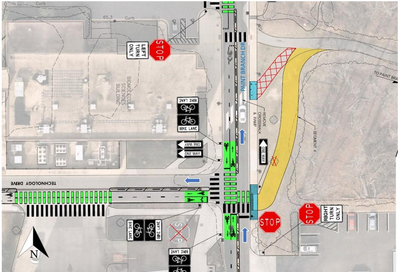
FIGURE 38: PROPOSED CONNECTION FROM PAINT BRANCH TRAIL TO TECHNOLOGY DRIVE
