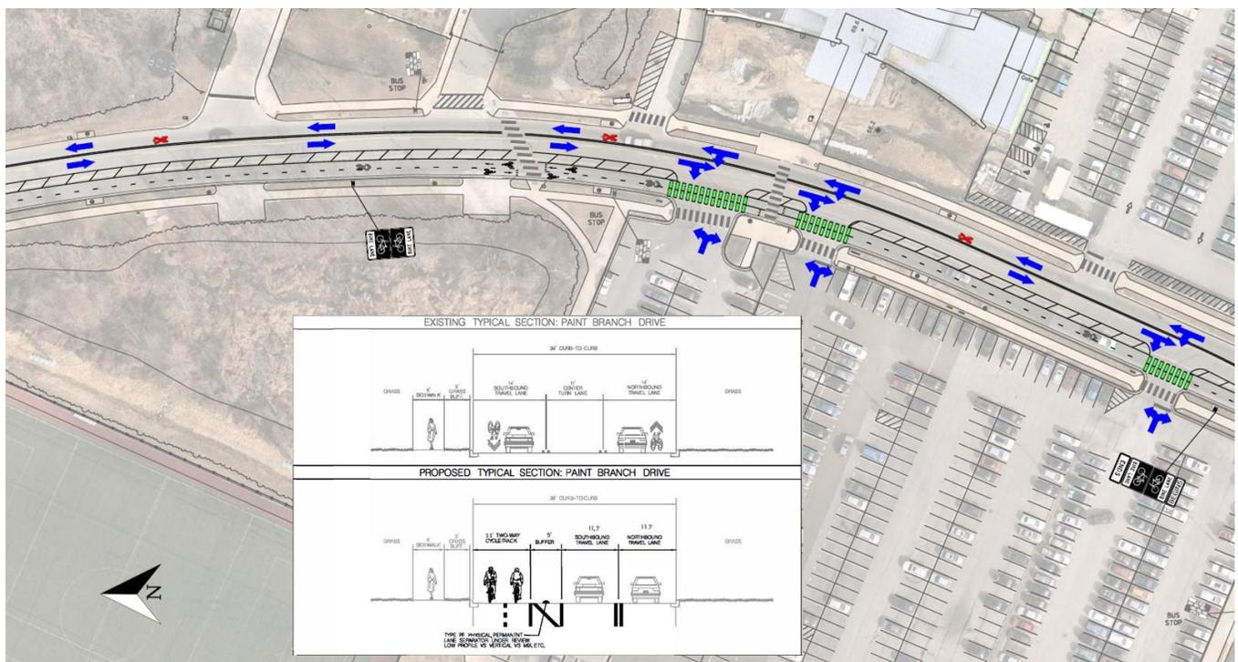
FIGURE 27: PROPOSED PLAN AND CROSS-SECTION FOR INTERIM 2-WAY CYCLETRACK ON PAINT BRANCH DRIVE
