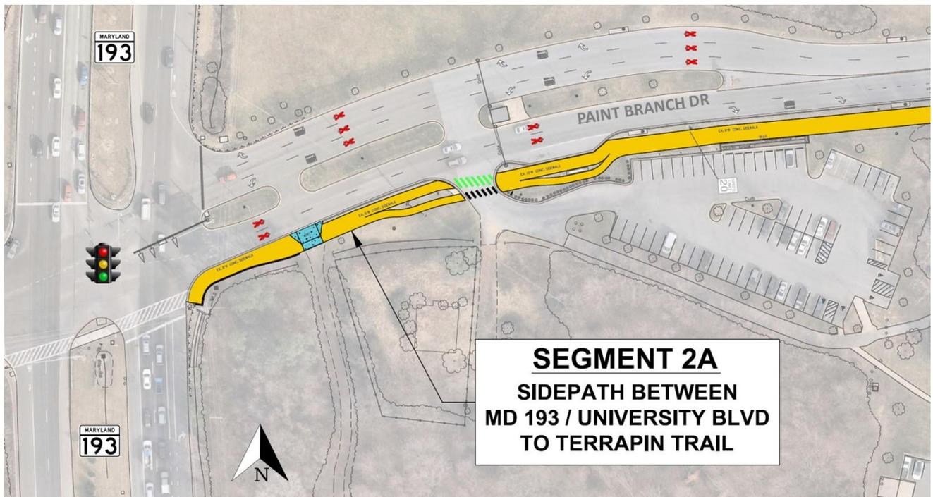
FIGURE 23: PROPOSED SIDE PATH ALONG SOUTH SIDE OF PAINT BRANCH DR NEAR MD 193
