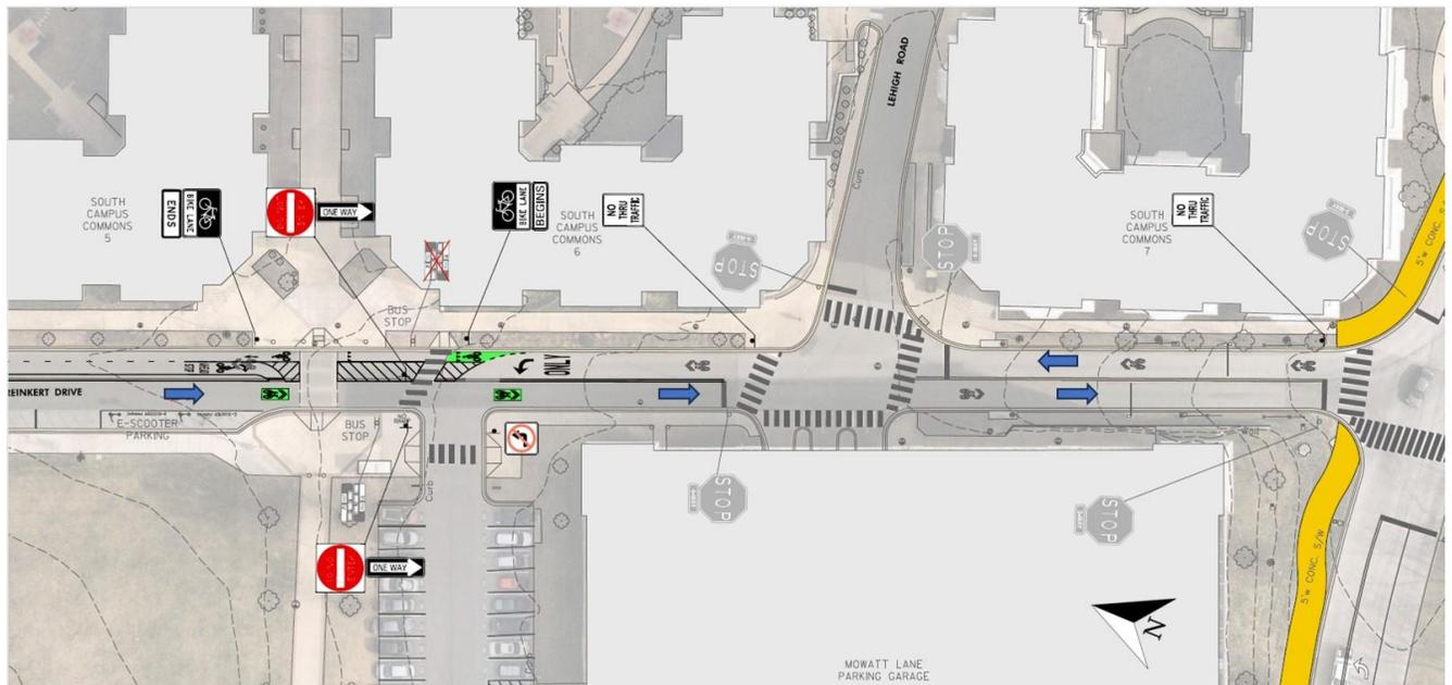
FIGURE 22: PROPOSED PREINKERT DRIVE CYCLETRACK TERMINATION AT MOWATT LN
