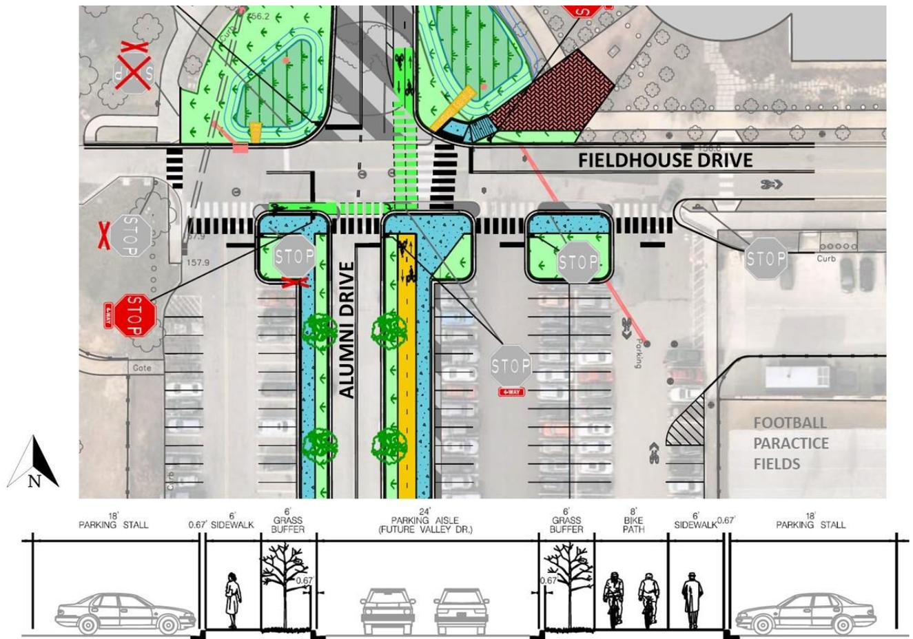
FIGURE 11: PROPOSED PLAN VIEW AND CROSS-SECTION VIEW OF ALUMNI DRIVE THROUGH LOT 1/Z, NORTH OF CAMPUS DRIVE
